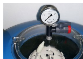
Optionally venting with Praher® S4 laboratory ball valve
