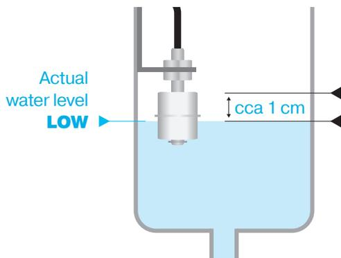
**Filling - ON** level at which refilling starts
