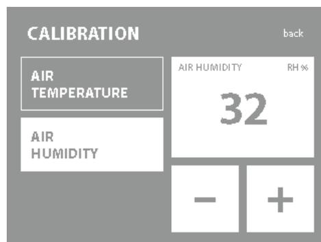
Calibration menu for air temperature and humidity
