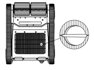
② Remove the plug cover. After fully charged, the plug should be covered back.
