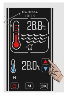
The actual pool water temperature is shown in the upper area of the display. The required temperature is shown in the lower area of the display. The required water temperature can be adjusted by touching the '**UP** / **DOWN**' touch button keys until the required temperature is displayed, adjustments are in  $0.1^{\circ}$ C increments.
