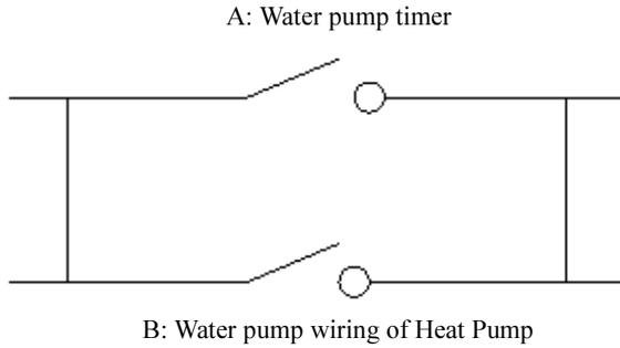
Note: The installer should connect A parallel with B (as above picture). To start the water pump, condition A or B is connected. To stop the water pump, both A and B should be disconnected.
