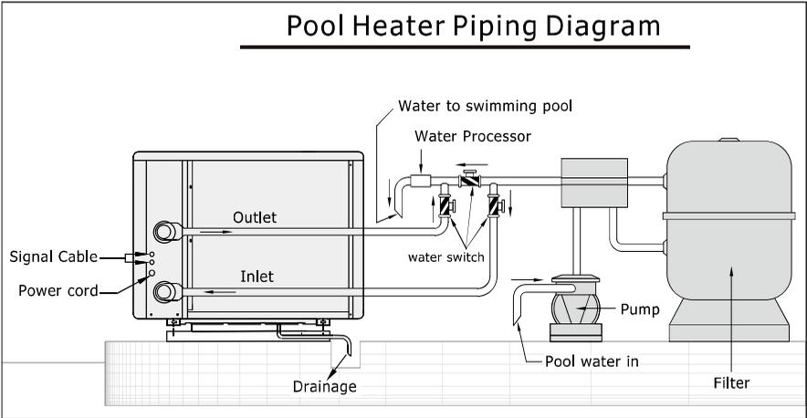
(Notice: The drawing is just for demonstration, and layout of the pipes is only for reference.)
