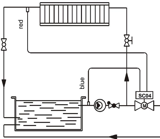
**When installing the sensors, make sure that each sensor is installed as close as possible to the medium to be measured (e.g., water)!**
