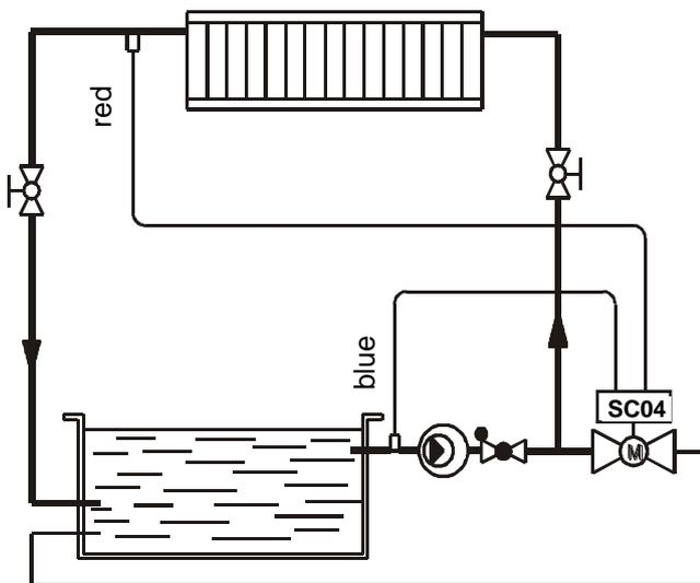
If the pool temperature drops by 1.5°C below the preset target temperature **[3]** and the collectable temperature rises by more than 4°C above the target temperature **[3]**, the device automatically switches to the heating position. RED LED **[2]** lit.
