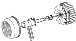
Check that the direction of motor rotation corresponds with that indicated on the specification plate (the fan should rotate in a **CLOCKWISE DIRECTION**, when viewed from the rear of the motor). If the motor is three-phase and it is observed that it is rotating in the opposite direction, then two of the supply phases should be inverted at the protection panel.
