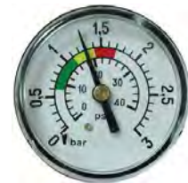
1,3 kg/cm 2 - 18,5 PSI: Proceed with Backwash operation
